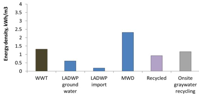
**Figure 5** Energy density of wastewater treatment (WWT) and other potable and non-potable water sources. Sources for energy density data WWT including conveyance were from (GEI Consultants and Navigant Consulting, 2010a); for LADWP groundwater, LADWP import, MWD and recycled water after secondary treatment were from (LADWP, 2011); for onsite graywater recycling using vertical flow wetland were from (Yu et al., 2013b).
