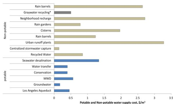
**Figure 7** Median potable and non-potable water supply option cost to LADWP (LADWP, 2011). The cost of graywater recycling was calculated based on gross treatment cost before factoring in water savings and the cost of retrofitting (Yu et al., 2013b).
