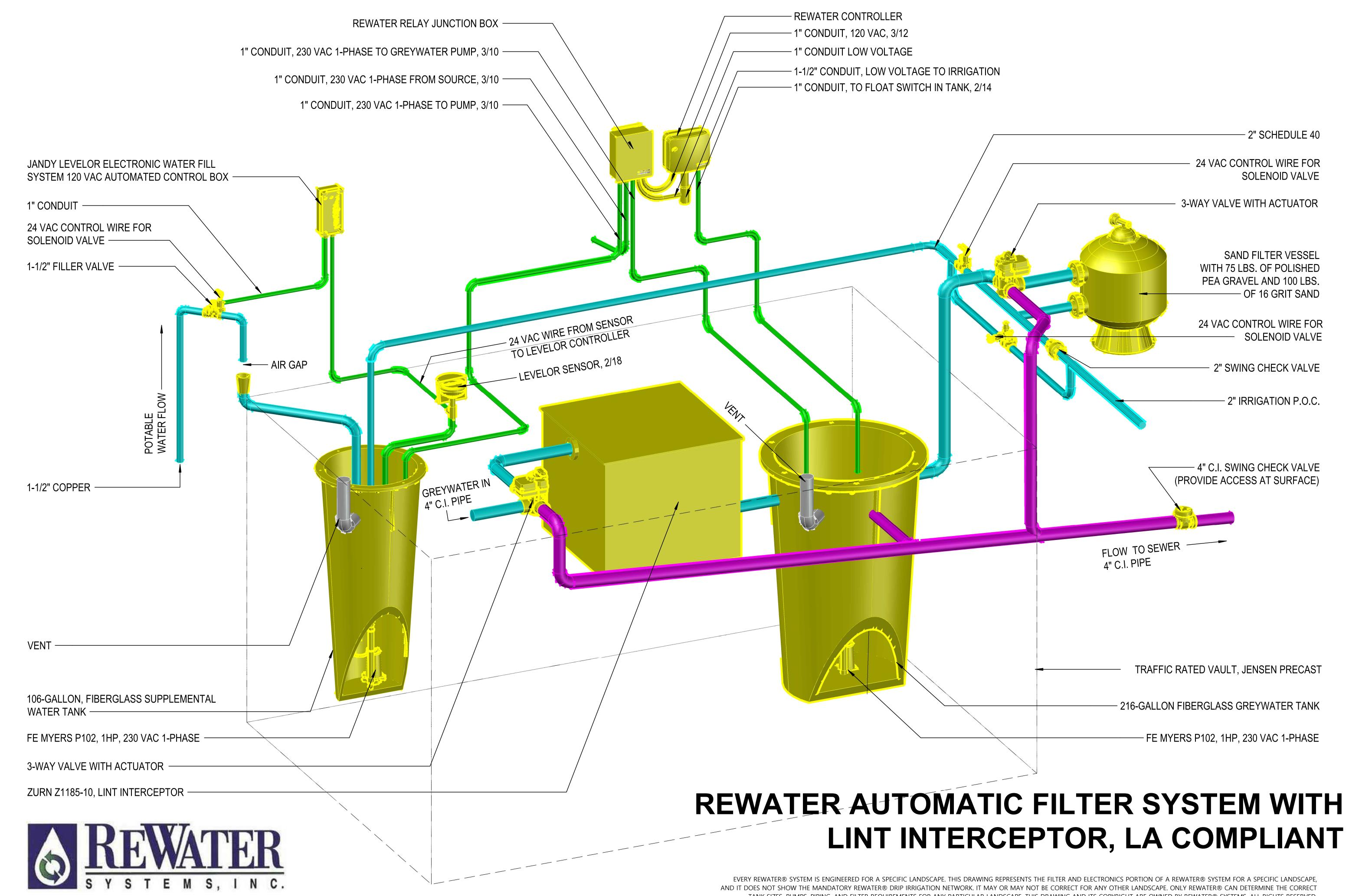
TANK SIZES, PUMPS, PIPING, AND FILTER REQUIREMENTS FOR ANY PARTICULAR LANDSCAPE. THIS DRAWING AND ITS COPYRIGHT ARE OWNED BY REWATER® SYSTEMS. ALL RIGHTS RESERVED
